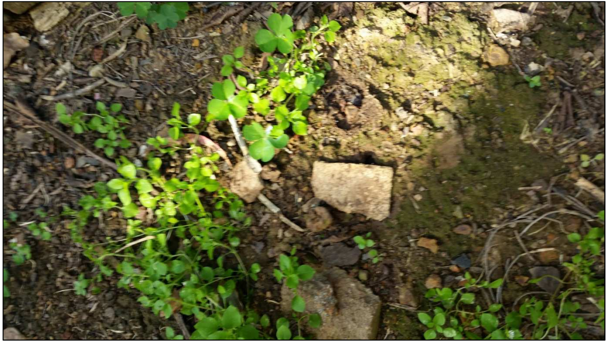
Photograph 7. Presumed asbestos fragments observed on northern side soil strip of 5 Station St.
